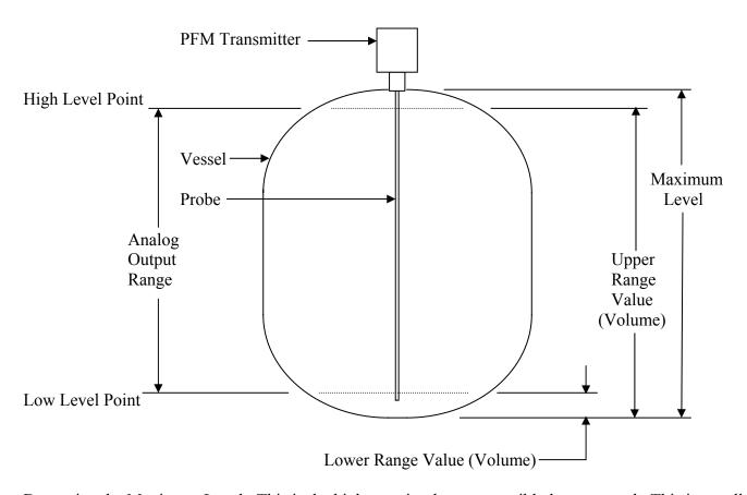
Determine the Maximum Level. This is the highest point that can possibly be measured. This is usually, but not always, the same as the tank height. Fill in the value below.
